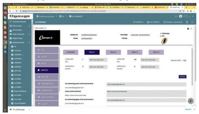
The Ogauge dashboard also offers live (realtime) monitoring of pressures, and trend analysis of relay operations and other parameters like suction and discharge pressures (when measured).
